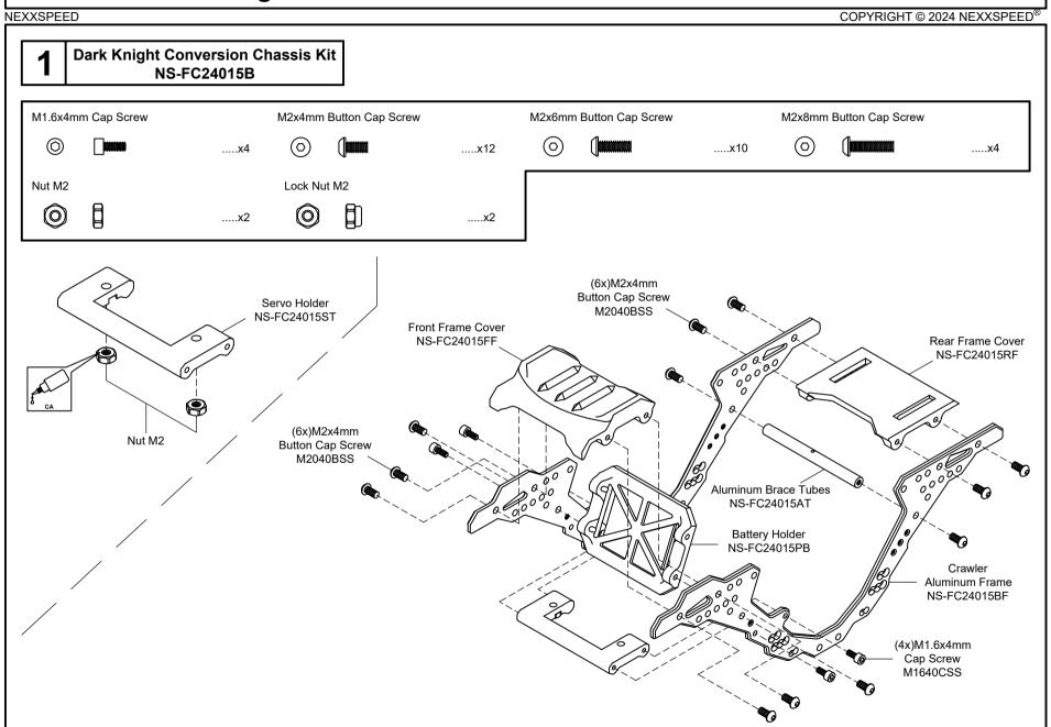
NEXXSPEED COPYRIGHT © 2024 NEXXSPEED® **Dark Knight Conversion Chassis Kit** NS-FC24015B Motor (Stock part (2x) M2x6mm not included) Button Cap Screw M2060BSS Servo (Stock part not included) Crawler Carbon Head ock Nut M2 NS-FC24015CC M2LN Right Frame Cover NS-FC24015FR (4x)M2x6mm Button Cap Screw M2060BSS Aluminum Skid Plate NS-FC24015FS (4x)M2x6mm **Button Cap Screw** (4x)M2x8mm M2060BSS **Button Cap Screw** M2080BSS
